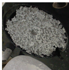
Unprotected and premature transom & outdrive zinc loss
