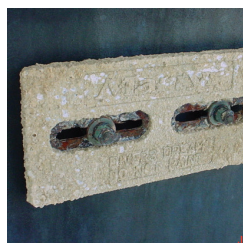
Unprotected and premature transom & outdrive zinc loss
